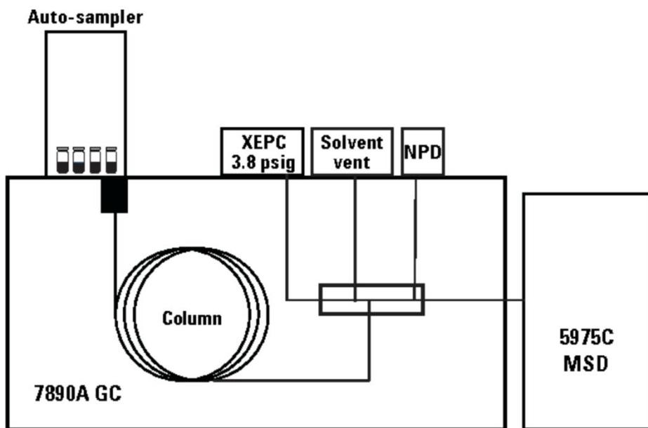
**Figure 1** GC/MS/NPD system configuration used for
